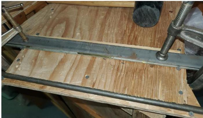
4. Fit this brass sides to the original plastic sides to see if the radius is what you want to match the existing skirt curve. Exact is not necessary as some variability existed in the real cars as it was done by craftsman, not machine.
